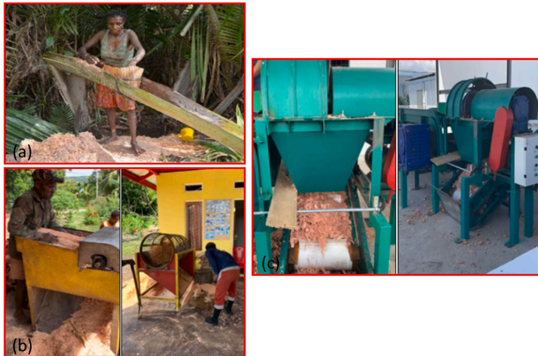
Fig. 2. Sago tree processing: (a) traditional process, (b) semi-modern process, and (c) modern process.
