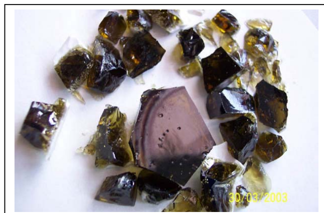
Figure 2: Melted slag produced by melting of rubber sludge
