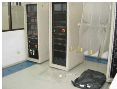
Figure 3 : Dynamic dilution with purified Nitrogen gas
